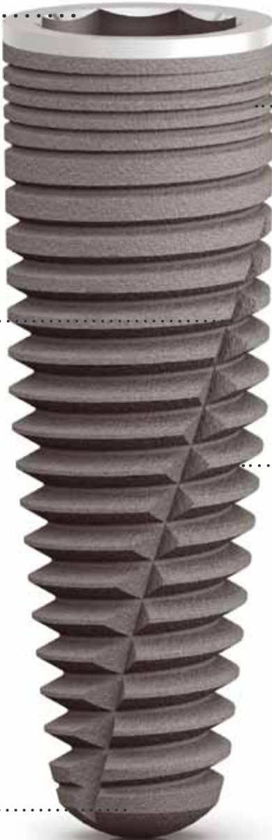
The coronal microthreading , has the same shape as the effective spire, but with a halved pitch. The microthreaded portion of the implant neck and the continuity of the main thread provide better primary stability.
