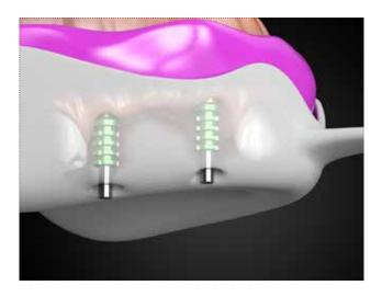
While waiting for the temporary or final bridge to be delivered, the abutments must be protected by PEEK caps (cod. SH-CG-ABU-F-380), that must be tightened at 9-10 Ncm.
