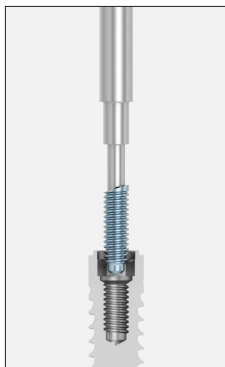
Figure 2. Broken screw during removal, hooked to the clutch drill
